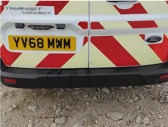
6: Bumper Rear Scratched Over 25mm Not Thru Paint
