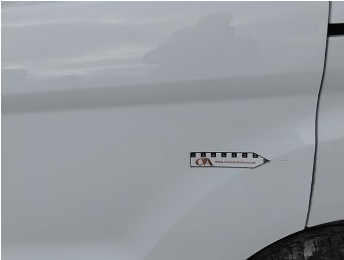
3: Door nsr Scratched UpTo 25mm Not Thru Paint
