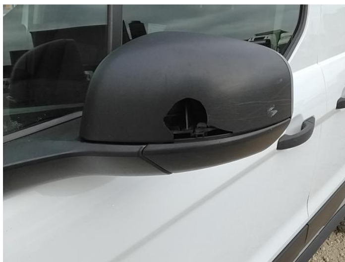
2: Door Mirror Assy nsf Broken Replace
