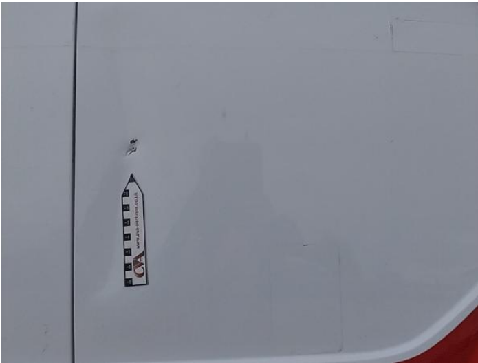
5: Door osr Dented With Paint Damage
