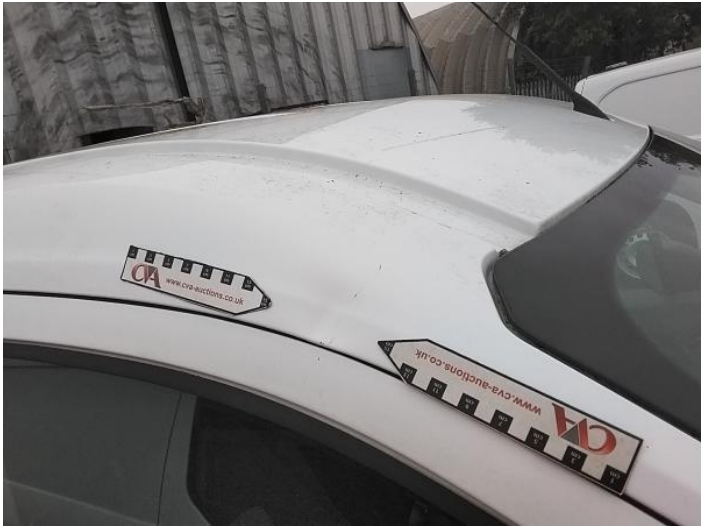
4: Roof Dented Over 30mm
