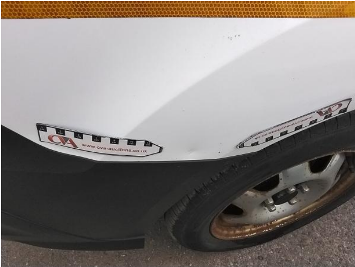
3: Qtr Panel osr Dented Over 30mm
