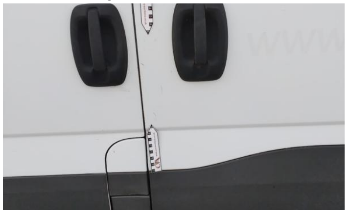
6: Wing nsf Dented With Paint Damage
