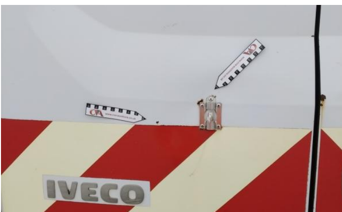
11: Panel Rear Scratched Rusted
