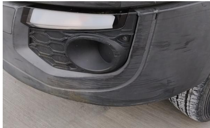
3: Bumper Front Cracked Over 25mm
