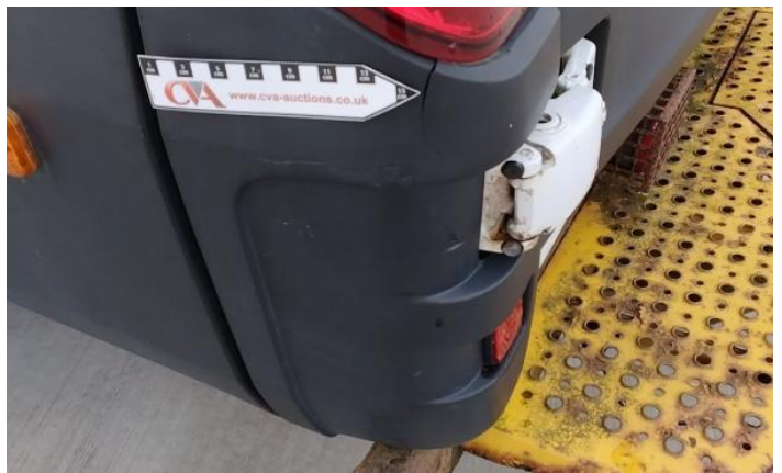
10: Qtr Panel nsr Rusted Over 5mm
