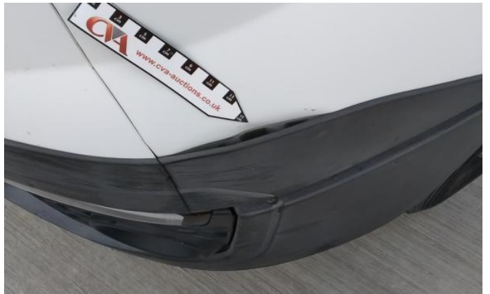
4: Bumper Front Chipped Over 5mm
